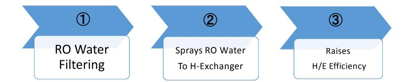
① Reverse Osmosis filter removes minerals and contaminants (cause of scale).
